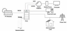
Stacked house BESS adopts modular design, the product is serial-connected through the battery module series to improve the system voltage and capacity, can match a variety of brands of inverters.
